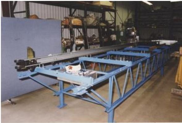
Main Spar table jig for NA337 rebuild
