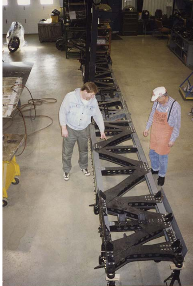
Note: George Roskopf (L) and Tom Mann ® with rebuilt Halifax main spar
